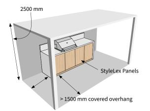
Note: If ceiling height is more than 2500mm, then the covered overhang should be increased accordingly.
